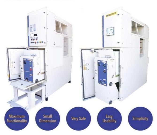
The PARAS panels consists of a withdrawable Air Insulated Vacuum circuit breaker, Instrument transformers, Protection relays with a full set of accessories, interlocks and with MS sheet enclosure. All the compartments are segregated by metallic partitions and the live parts are Air Insulated. The panel is modular in construction, which allows additional panels to be lined up beside each other to form a switchboard, interconnected by busbars.
